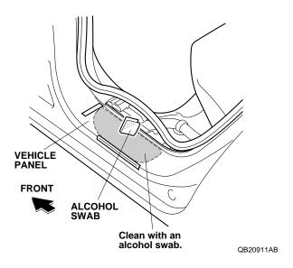
24. Align the left rear door sill trim with the masking tape and install the left rear door sill trim to the vehicle panel.
