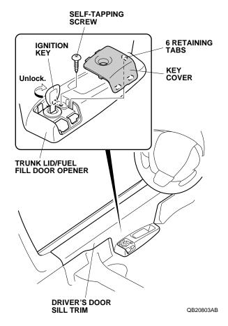
3. Remove one self-tapping screw from the trunk lid/ fuel fill door opener cover.
