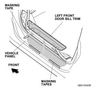
15. While applying light pressure against the left front door sill trim, carefully remove the adhesive backings.
