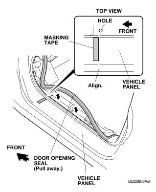
9. Attach a piece of masking tape to the vehicle panel in the location shown.
