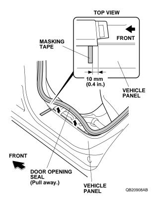
Attach a piece of masking tape to the vehicle panel in the location shown. 20. Align the left rear door sill trim with the masking tape attached in step 19, then attach another piece of masking tape to the vehicle panel along the outside of the left rear door sill trim. Do not tape down the left rear door sill trim.
