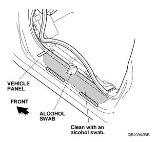
14. Align the left front door sill trim with the masking tape and install the left front door sill trim to the vehicle panel.
