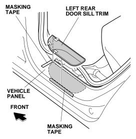
25. While applying light pressure against the left rear door sill trim, carefully remove the adhesive backings.
